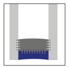
Ködispace 4SG forms a chemical bond with the glass and with the silicone seal.
