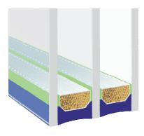
The traditional Insulating Glass construction uses frames of rigid spacer profiles which are filled with desiccant, coated on both sides with butyl and then placed on the glass and then finally sealed with secondary sealant.
